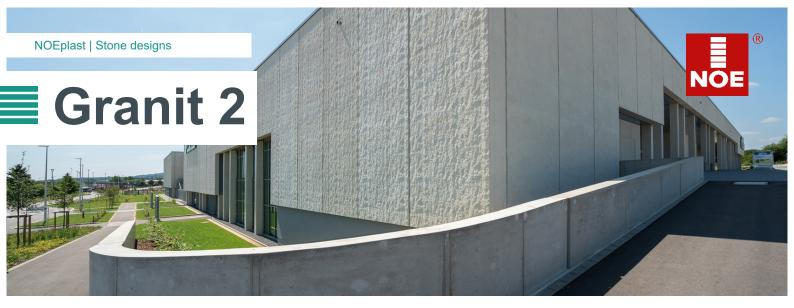
This textured formliner gives the concrete the appearance of a large granite panel with a coarsely worked surface. The design of the formwork should take into account the orientation of the texture on the formliner.
