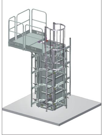
The NOEtop FS allows columns with cross sections from 200 to 600 mm to be concreted without tie rods. The cross sectional dimensions are adjustable in 50 mm increments.
