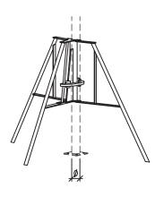
Folding tripod for Ø 48- 90 mm Part No. 900072 Folding tripod for Ø 90-120 mm Cantilever slab 450 mm Consisting of cantilever girder support (Part No. 115434), cantilever slab 450 mm (Part No. 115435) and spanner bolt R12 (Part No. 319341 — 2 No)
