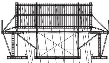
Use as box-section formwork
