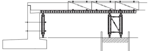
Use as tunnel formwork
