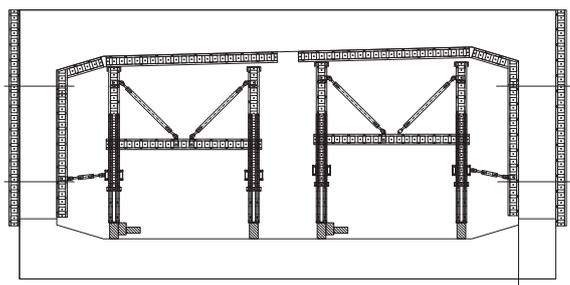
Use as integrated travelling formwork
