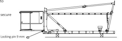
Fit lifting dog for erecting the formwork and attach crane rope to lifting dog. Lift slowly with the crane and move to the point of use.
