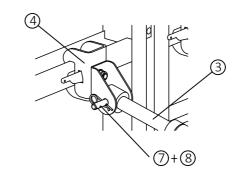
Detail C: Attachment to base support plate
