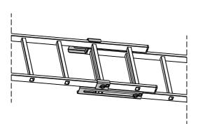
The ladder on the long side piece can now be moved in the elongated hole of the ladder extension.
