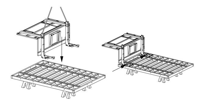
Use the clamping jaw to mount 2 buffer supports in the bottom top-hat profile, and secure by driving in the wedge,
