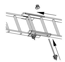
◆ Thread the ladder into the ladder extender piece, guide the tie rod through the hole and secure with the Sprint nuts.
