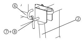
Detail B: Attachment to formwork
