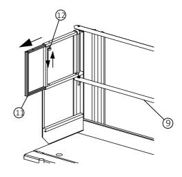
◆ To close the side guard rail release the screw, retract the extension, fold the side guard rail onto the rear guard rail, and re-tighten the screw to secure.
