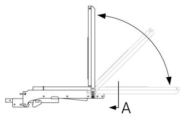
• Pull on the pin to open, and fold out guard rail. Then release pin so that it closes and re-engages.
