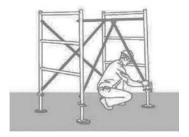
◆ Attach a diagonal and K-diagonal to the long sides, securing them to the base jack.
