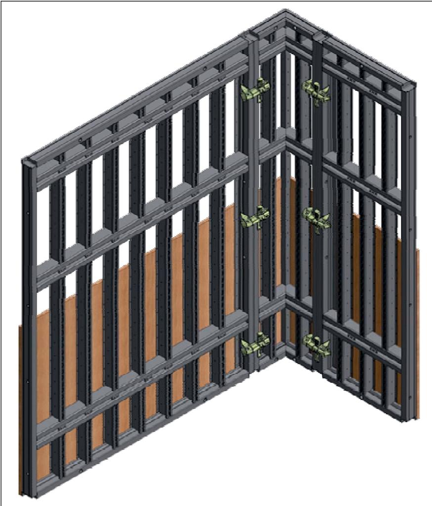
NOEtop R considerably extends the range of use of the NOEtop formwork system. Top hat profiles with plastic strips are integrated into the frame panels with integrated bracing members. This allows the formwork facing to be attached irrespective of the panel layout.
