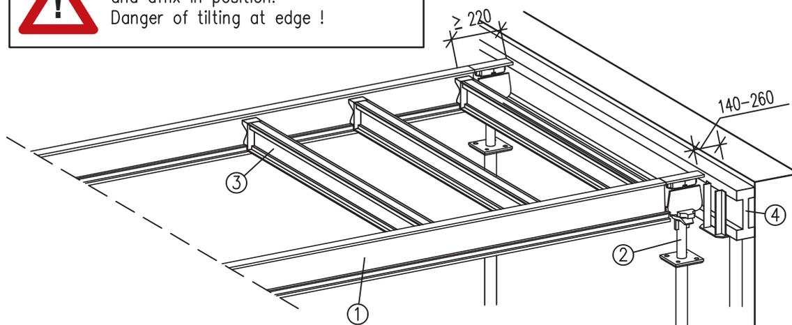
If the NOEdeck drophead is positioned directly against the wall, check that it is possible for the facing to project.
