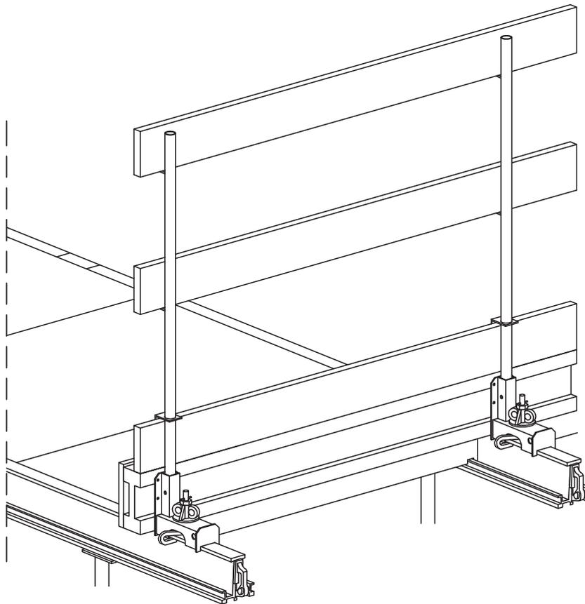
The handrail tube holder be slid along the aluminium longitudinal girder as required. With the help of the Sprint, it is clamped firmly in place on the girder.
