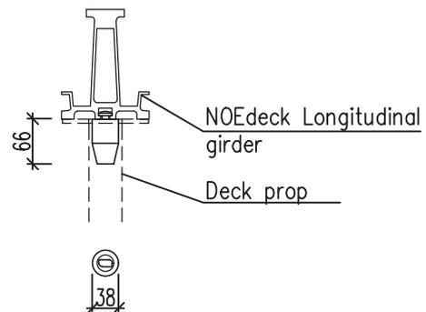
For attaching deck props to a NOEdeck longitudinal girder.
