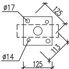
Mounting on ADS support or NOEprop with 2 M16x40 Part No. 313400
