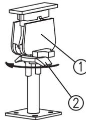
Drop piece top, strike the tie plate clockwise and lock it.
