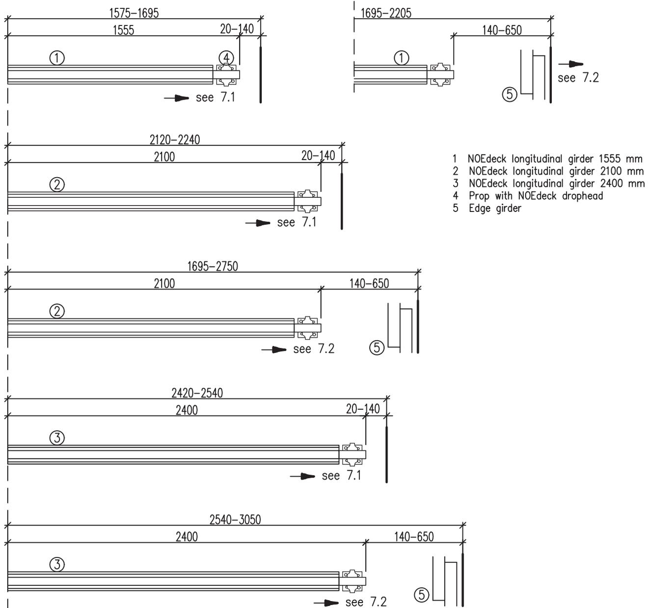
A residual distance of 3050 mm to 3130 mm (= 2x1555+20 mm) cannot be filled using the solutions shown above. In this scenario, the residual distance must be reduced by selecting another arrangement of girders or the series of girders must be joined at another position.
