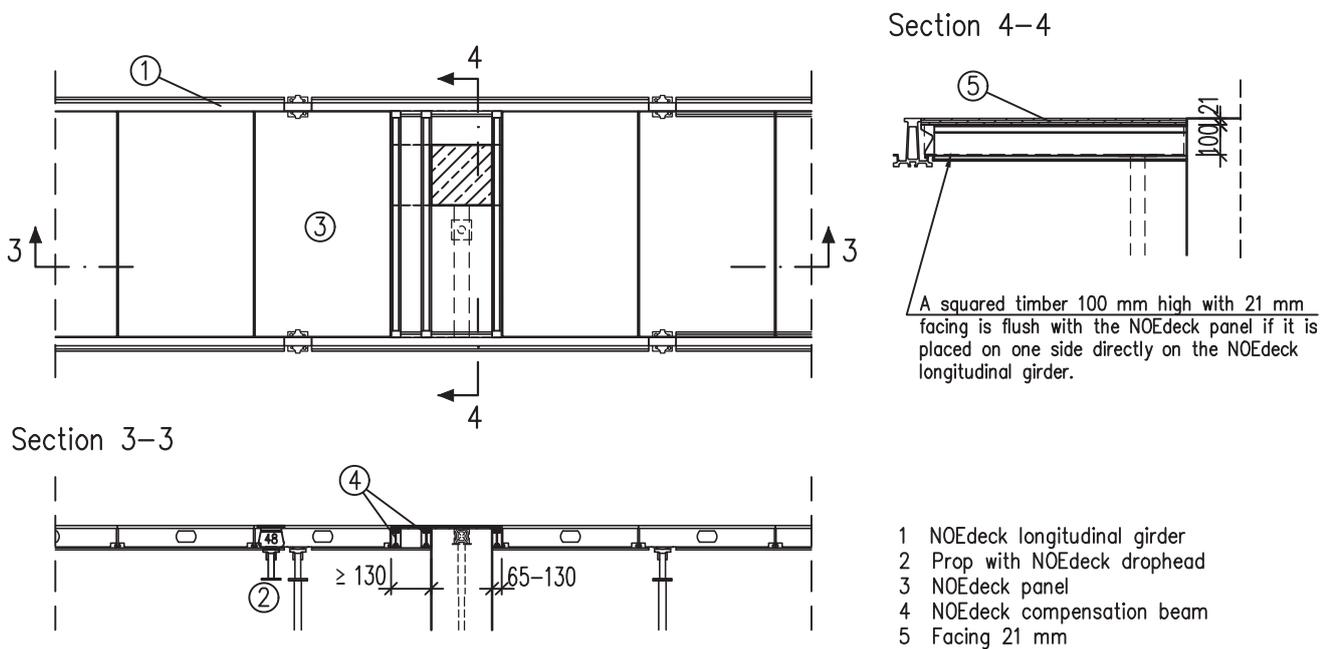
Depending on the arrangement of the NOEdeck panels, one or more NOEdeck compensation beams can be positioned to the side of the columns. The propping requirements for the area of deck near the column depend on the deck thickness and the loadbearing capacity of the facing used at the residual area.
