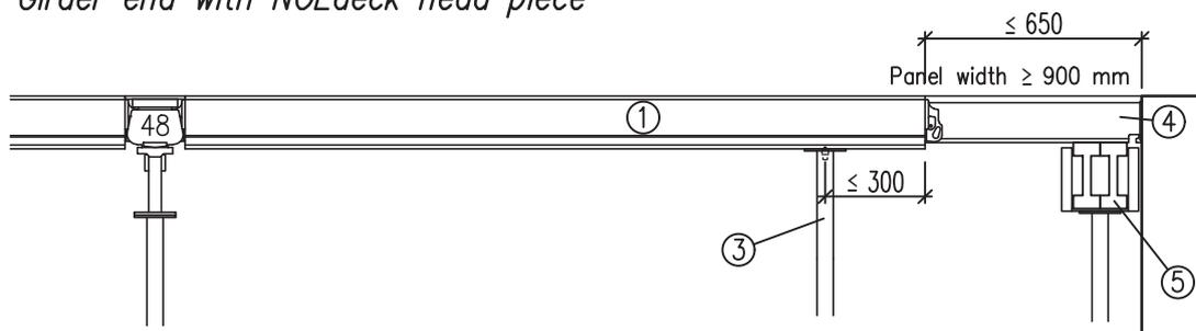
For residual distances of 140 to 250 mm the H20 girders cannot be placed at an angle; they must be aligned in a row.
