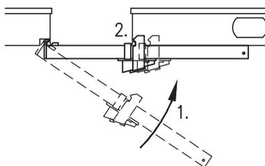
1. Suspend the fixed end of the compensation bridge in the NOEdeck panel or longitudinal girder and swing the compensation bridge upwards.
