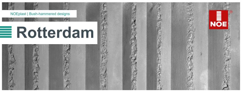
A concrete panel moulded from triangular timber laths placed adjacent to one another provided the basis for the Rotterdam textured formliner. The apexes of the concrete triangles were then tooled flat.
